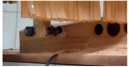
Milling into the speaker cut-outs
