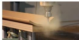
Levelling the lower edge of the standing surfaces
